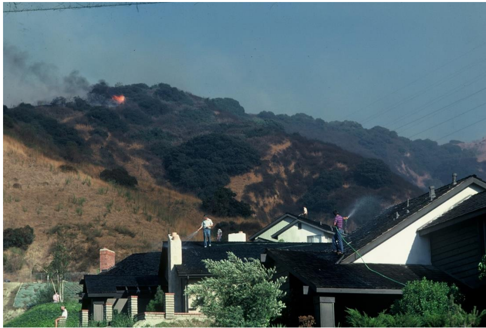
1978- Three people watering the roofs of their wood-roof community while they still have water pressure. Two people are watching on the ground. Backyards are planted with low-fuel plants, protecting the uphill facing sides of the homes from direct flame impingement. Little good will this do when firebrands start raining down on the roofs as the wind shifts..
