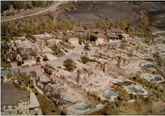
1999 – Crest De Ville Fire – A small fire quickly destroyed a new wood shingle roof community despite available water.
