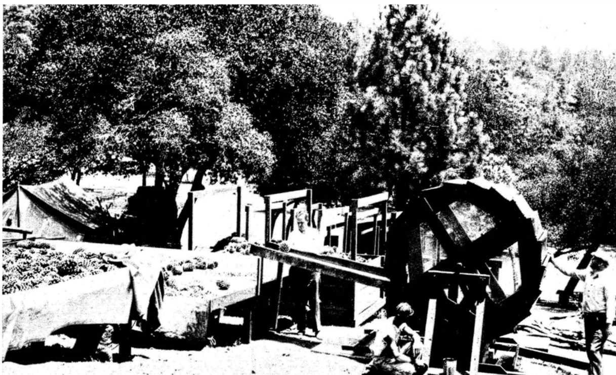
Photo 7: Henninger Flats Nursery July 20, 1929. Cone extractor for Coulter pine ( Pinus coulteri ) is shown on right and drying flats on left. Roger Bodine on left.
