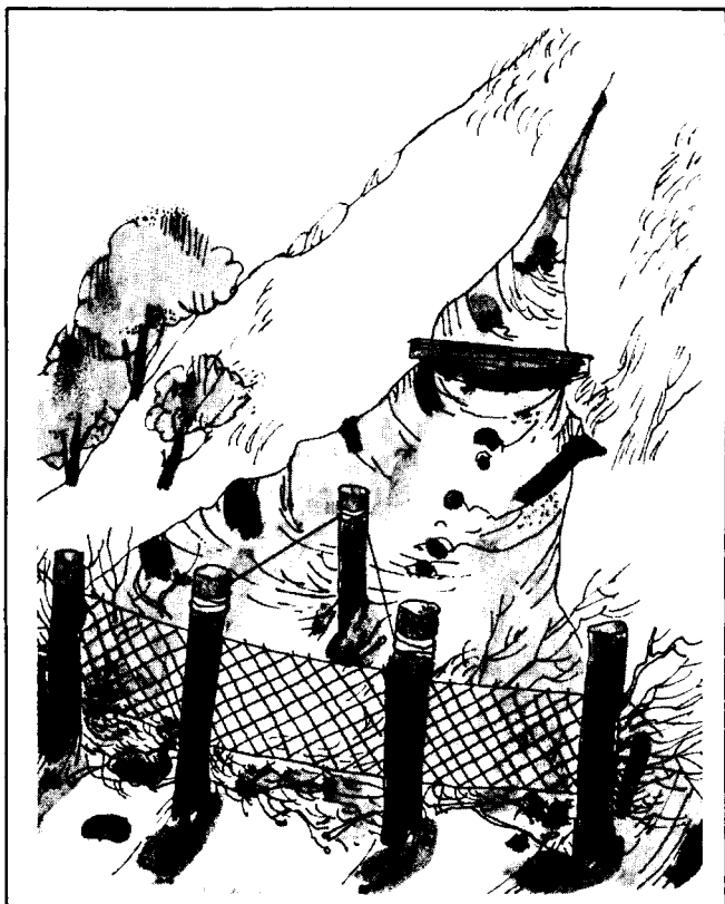
Figure 27 —Check dams can reduce gully erosion.
