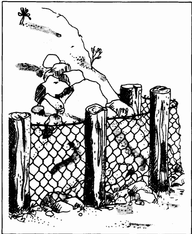
Figure 30 —Chain-link fences stop rocks, even large boulders.
